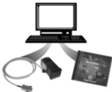
**N.B.:** RS232 interface for PC configuration è fornito is supplied with WINSTRUM programming software. make the connection with the device powered and with inputs and outputs disconnected.
