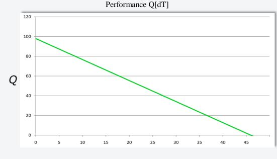
dT  $dT^{\circ}C = T^{\circ}$  ambient - T° internal Q - cooling capacity, W. for ambient temperature +35 ° C and rated voltage
