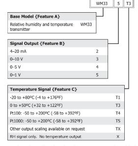
To construct the order code, select the relevant feature from the tables below, starting with the base model, which is {Feature A} and then add on options to create a string: {Feature A}+{Feature B}+{Feature C}+{Feature D}+{Feature E}+{Feature F}
